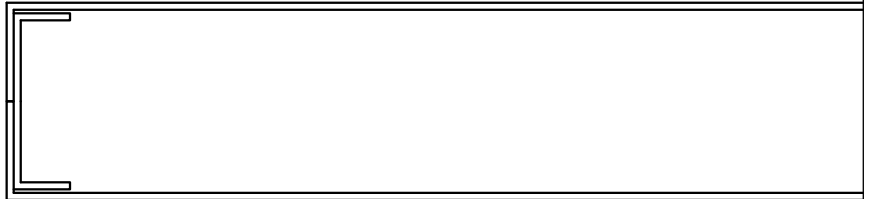
Butted Square Edge with "U" side channel
