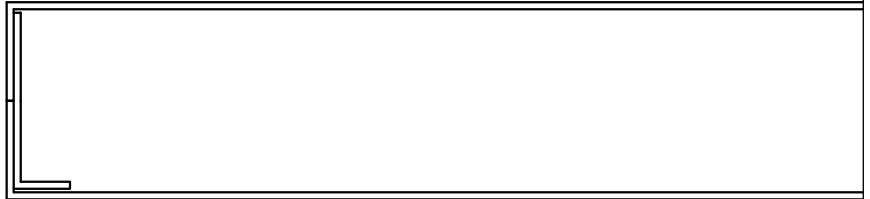
Butted Square Edge with "L" side channel
