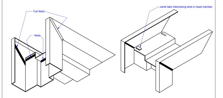
All elements of the frame member are continuously welded
